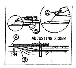
DOUBLE CHECK THE POSITION OF SAFETY SWITCH WHEN THE POWER IS ON, THE TRIMMING KNIFE SET MUST BE IN ITS SET POSITION.
